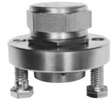
WD450 Thermodynamic Steam Trap Module (Top Mount Style) Recommended for horizontal piping installations only so that cap can be oriented upwards as shown.
