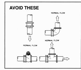
The W Series check valve installs between two pipe flanges. The body is flangeless and is centred in line by the surrounding flange bolts.
