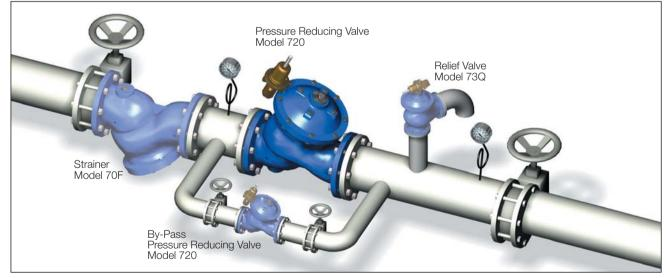
In addition to the Model 720 Pressure Reducing Valve, BERMAD recommends that the system also include:
