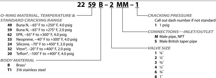
† For PED applications, brass bodies are limited to a maximum temperature of +100° F (+38° C).
